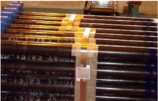
Image 7 – polypropylene overlapping technique
