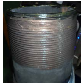
Figure 13.10.7.3 – Thread Compound (Plug)
