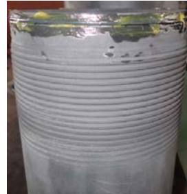
Figure 13.10.7.1 – O-ring fitted (Plug)
