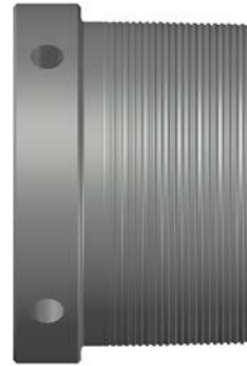
Figure 13.5.1 – Example of main body for lift plug (seal removed)
