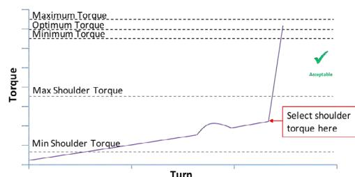
Figure 12.1.3 – Example of an acceptable JFELION/JFETIGER make-up graph (the maximum torque value of the dope hump exceeds the maximum shoulder torque, however linearity is re-established prior to shouldering at a value below maximum shoulder torque)
