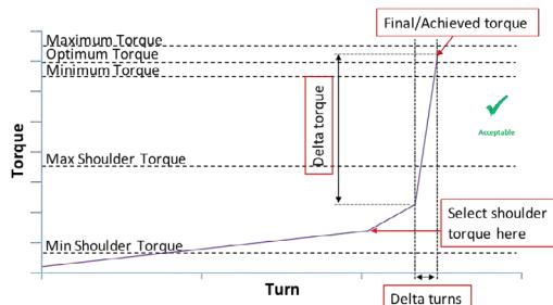
Figure 12.3.2 – Example of an acceptable FOX make-up graph (Shoulder point is below maximum shoulder)
