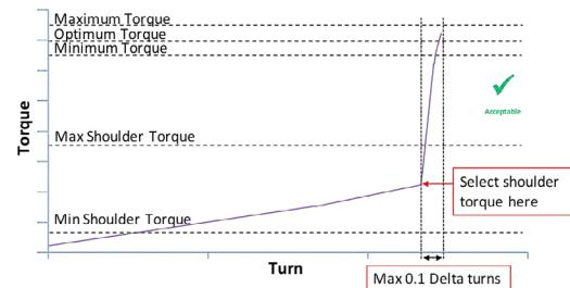
Figure 12.1.5 – Example of an acceptable JFELION/JFETIGER make-up graph. Minor slippage during thread engagement and slope returns to similar gradient once slipping occurs. Rectify for next make-up
