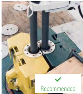
Using a dual completion tong eliminates the requirement for a spreader bar
