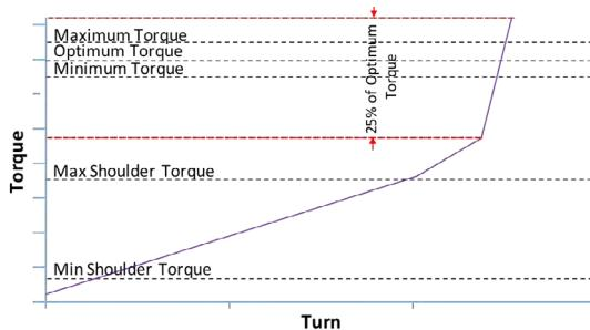
Depending on the type of locking compound, connection size and wall thickness, increasing the make-up torque may be required. The MTS (Maximum Torque with Sealability) value can be utilised in situations where there are concerns the shoulder torque or make-up profile will not be acceptable. If selecting to utilise the MTS figure, the torque window should be set as follows:
