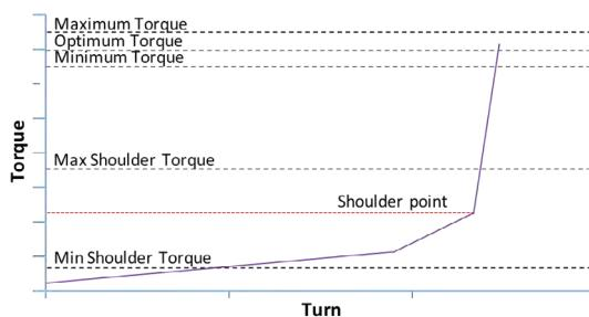
If the shoulder torque is above the maximum allowable, 25% of optimum torque should be applied after shouldering. This can result in the final torque exceeding the recommended maximum torque for the connection. An example of a JFEBEAR TT graph is shown below where the recorded shoulder torque is higher than the allowable maximum shoulder torque during thread lock make-up.
