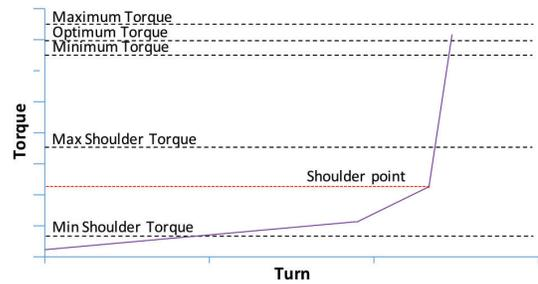
If the shoulder torque is above the maximum allowable, 25% of optimum torque should be applied after shouldering. This can result in the final torque exceeding the recommended maximum torque for the connection. An example of a JFEBEAR TT graph is shown below where the recorded shoulder torque is higher than the allowable maximum shoulder torque during thread lock make-up.
