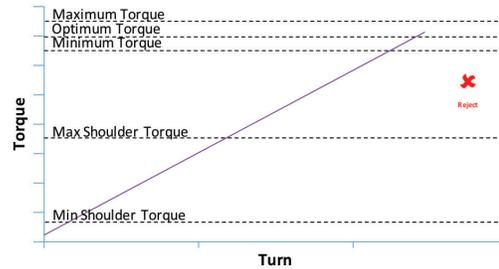
Possible causes of the unacceptable graph profile but not limited to, are as follows:
