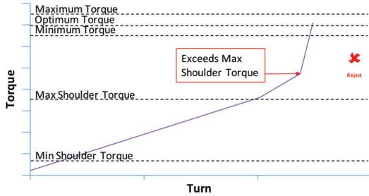
Possible causes of the unacceptable graph profile but not limited to, are as follows:
