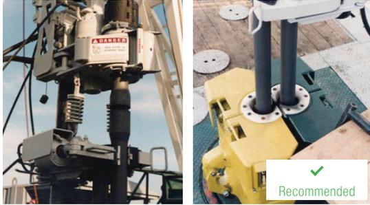
Using a dual completion tong eliminates the requirement for a spreader bar
