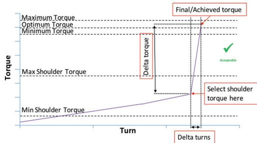
If a case exists where premature dump torque occurs or a high shoulder is observed, if:
